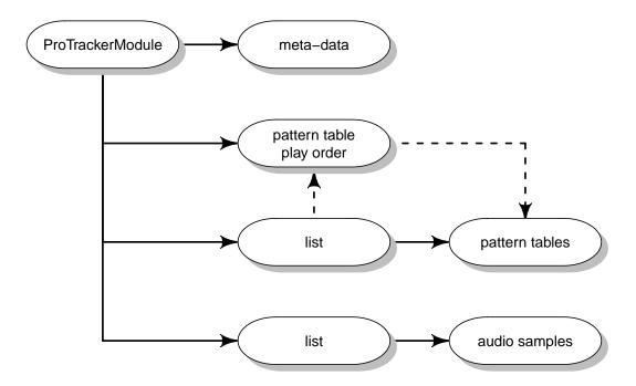
This class is designed to hold all relevant information of a ProTracker module (MOD) for which ProTracker 2.3a documentation was used. The ProTrackR package may be compatible with earlier or later versions, but this was not tested. Use read.module and write.module to import and export objects of class PTModule.
