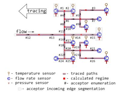
In latter case no more than two nodes must be equipped with pressure and temperature sensors
