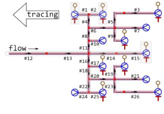
In latter case no more than two nodes must be equipped with pressure and temperature sensors whereas for other nodes only flow rate sensors must be installed.
