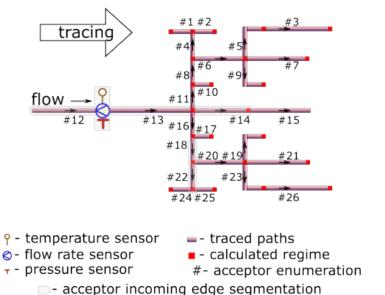
Tracing starts from sensor-equipped root node and goes forward, i.e along the flow direction. Function m325traceline serves under the hood for tracing identified linear segments from root node to every terminal node. Hence they only need root node to be equipped with sensors. Sensors at other nodes are redundant in forward tracing, since the tracing algorithm by no means consider them for tracing.
