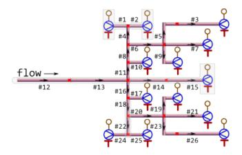
As it may be seen from the figure there is a particularity in topology of the provided directed graph: each node has only single ancestor. Hence one of isomorphic representation of such directed graph is a data. frame in which each row describes a node along with its incoming edge and each column contains an attribute value for that node or an attribute value for its incoming edge.
