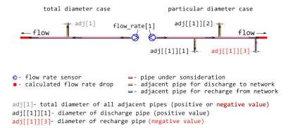
Usually, there are no additional sensors that could measure flow rate in each flow fork. In that case they only may operate with geometric factors, i.e. assuming that flow rate is proportional to square of pipe diameter.
